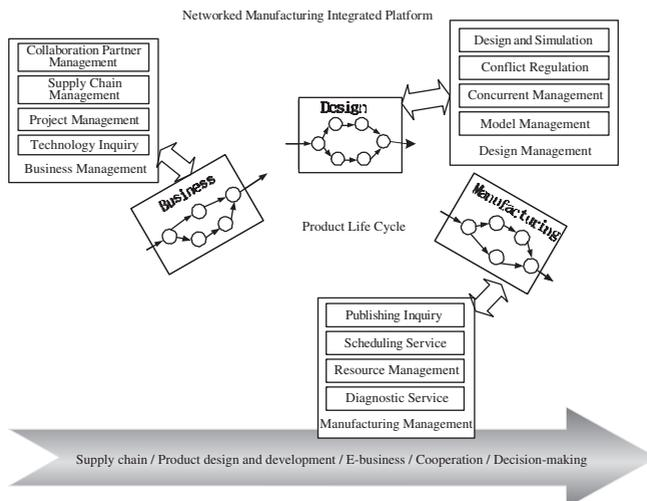
Figure 4. The operation of networked manufacturing aided by the NMIP.
