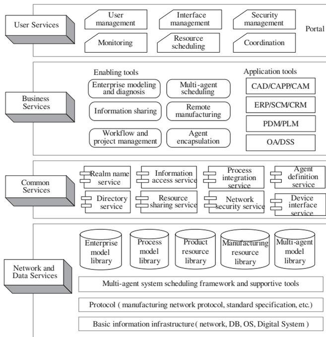
Figure 5. NMIP architecture based on a multi-agent system coordination control framework.
