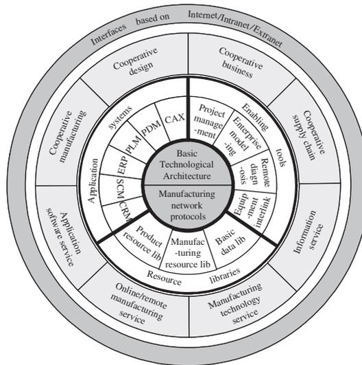
Figure 2. The architecture of networked manufacturing. The levels from inner to outer: Core level; Software and enabling tools level; Applications service level; User level.
