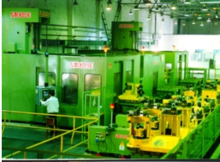
Figure 4.2 FMS for oil well drill production
